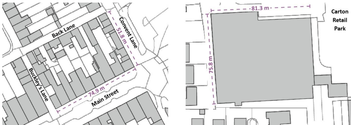
Figure 4.12 A Comparison of Block Sizes and Urban Grain in Maynooth Town Centre
